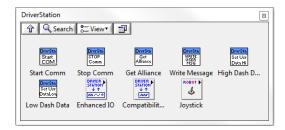
The Driver Station VIs can be used to relay information from the robot to the laptop, check the battery power of the robot, set the controls of the robot based on the current competition mode, and display information from the outputs you define. For more information, see the <u>Dashboard Coding</u> tutorial
