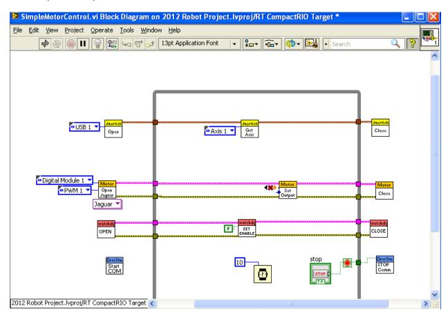
Remove the broken wires by going to **Edit»Remove Broken Wires**. Next, connect the **value** output from the joystick Get Axis VI to the **speed** input of the PWM Set Speed VI. Finally, close the joystick reference with a Close VI.
