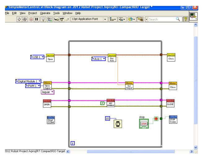
Click the run button to download the VI to the cRIO. Once the code downloads, move the joystick forwards and backwards to move the motor with varying speed and direction. Press the stop button when finished.
