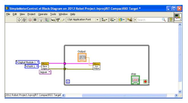
Finally, place the **Close** VI from **WPI Robotics Library»RobotDrive»Advanced»Motor Control** palette to the right of the while loop and then wire the **reference** and **error** outputs of the Set Speed VI to the inputs of the Close VI.
