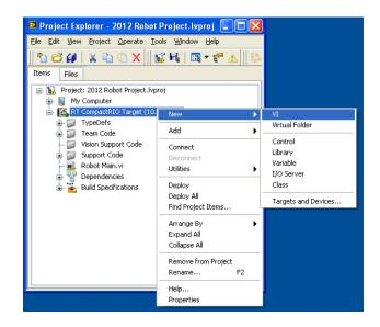
Save the new VI as *Simple Motor Control*. Notice that LabVIEW places the new VI inside the cRIO target tree, which means the VI will run on the cRIO.
