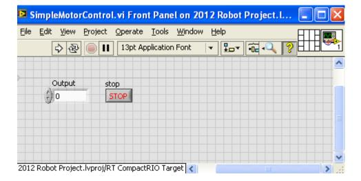
Once the program has finished downloading, try changing the value of the speed control from 0 to 0.1. The motor should now start moving slowly.
