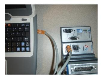
Power the driver station and configure it using your team number (See the FRC Driver Station Tutorial). This will set up the IP address of the driver station and the computer.
