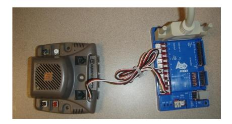
Next connect the motor to the M+/M- terminals on the Jaguar controller. Red is positive and black is negative. Now connect the Jaguar motor controller's V+/V- terminals to the 12 volt battery through the power distribution board. The controller fan should also be connected to the V+/V- terminals to prevent overheating. Before continuing make sure the fan is on and that the motor is secured so that it does not move while running.
